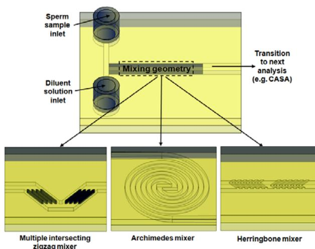
**Figure 4. Schematic diagrams of a microfluidic device and three candidate geometries of micromixers (multiple intersecting zigzag, Archimedes, and herringbone) for mixing of sperm with a diluent solution for activation and delivery to CASA.**
