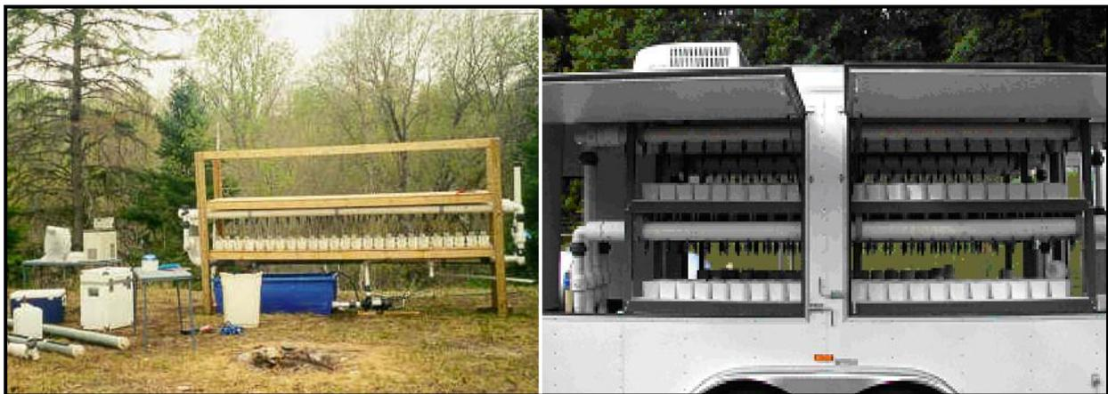
**Figure 1. Portable egg incubation systems. Left) a prototype system that could be transported to a riverside location for on-site fertilization trials to evaluate cryopreservation treatments. Right) a self-contained, temperature-controlled, recirculating system built on a trailer that can be disinfected and transported for cryopreservation experiments.**
