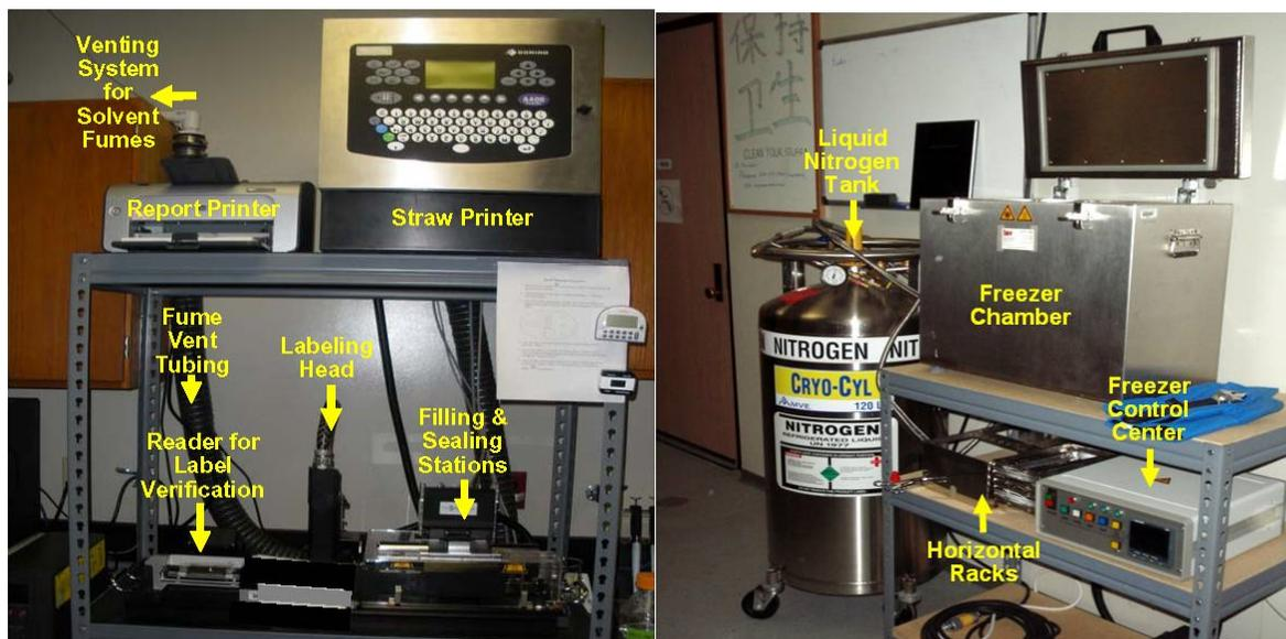
**Figure 1.** In the MAPI system (left), sperm suspensions are loaded and packaged into straws at filling and sealing stations, labeled under the labeling head driven by the straw printer, and pass a barcode reader for label verification. Next, the straws are laid on horizontal racks and placed in a programmable freezer (right) controlled by regulating liquid nitrogen flow from a pressurized storage tank. To see MAPI in action, [click here](#).
