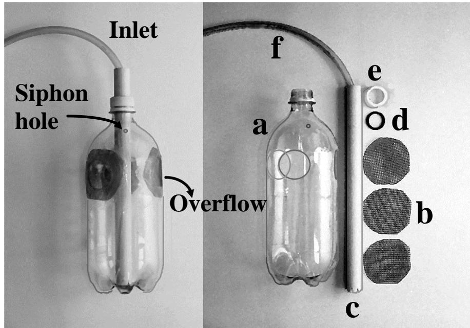
**Figure 1.** Assembled jar and components for the incubation of fish eggs: 3-L plastic bottle (a); circles of nylon screen (b); 1.91-cm PVC inlet pipe (c); 1.91-cm rubber gasket (d); original plastic bottle cap (e); plastic tubing of variable length for water inlet (f). Note the five protuberances (feet) on the base of the bottle which ensured even distribution of water. Figure reprinted with permission of the American Fisheries Society (Glenn and Tiersch 1997).
