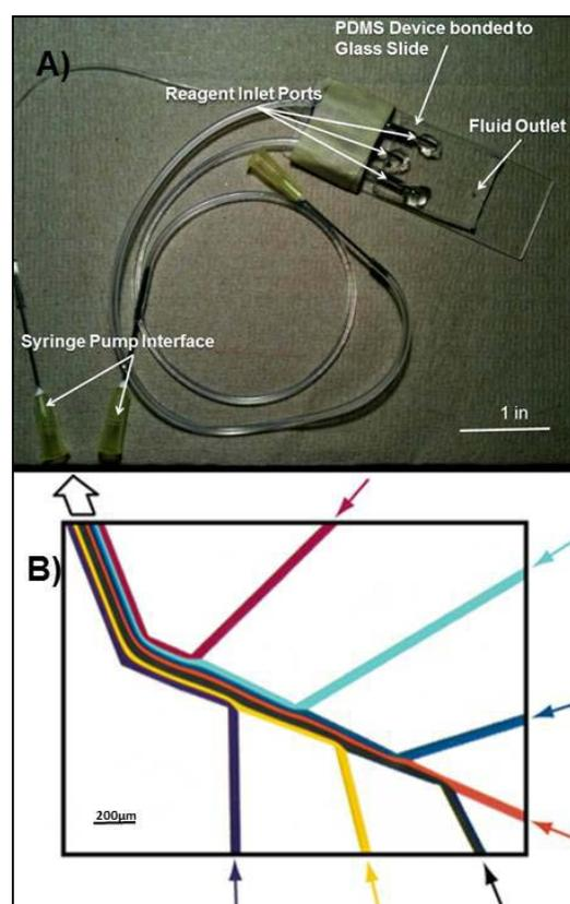
**Figure 1. A)** Example of a microfabricated chip for sperm analysis, whereby sperm samples are introduced into the microfluidic network through small-bore Tygon tubing. **B)** Example of laminar flow in a microfluidic network designed by Whitesides and colleagues, where inlet streams of dyed water do not mix. Image in (B) from *Science* cover (2 July 1999) reproduced with permission from AAAS.
