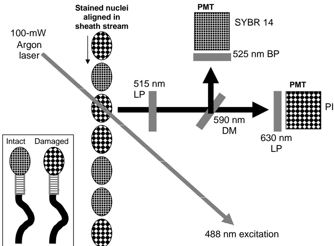
**Figure 1.** Schematic representation of the flow cytometric evaluation of sperm for intact plasma membranes (SYBR 14 positive) and compromised membranes (propidium iodide (PI) positive). The analysis requires the use of long-pass (LP) and band-pass (BP) filters as well as a dichroic mirror (DM) for detection of stained sperm by specific photomultiplier tubes (PMT).
