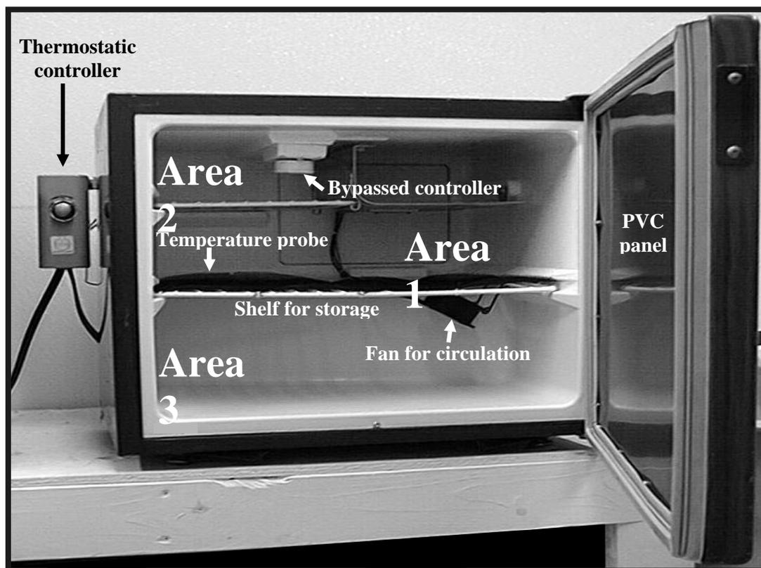
**Figure 1. Front view of a modified incubator equipped with external hydraulic-action thermostatic controller mounted on the side. A sensing bulb and capillary tubing were inserted through a hole in back, and attached above the center shelf. The three areas indicated were used to measure temperature variation.**
