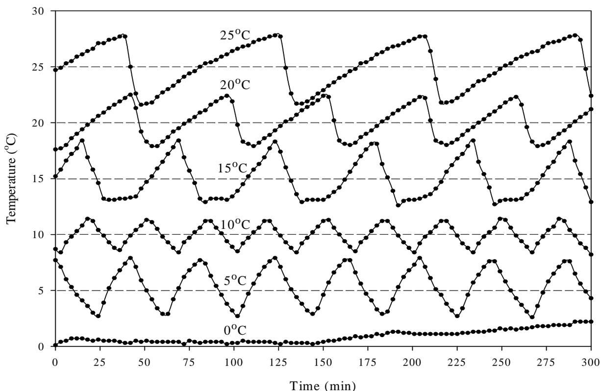
**Figure 3. Temperature variation in modified incubators at six temperature settings (0, 5, 10, 15, 20, and 25 °C). A type-T thermocouple and data logger were used to record temperatures at the center of the middle shelf. Ambient room temperature (AT) was also recorded.**
