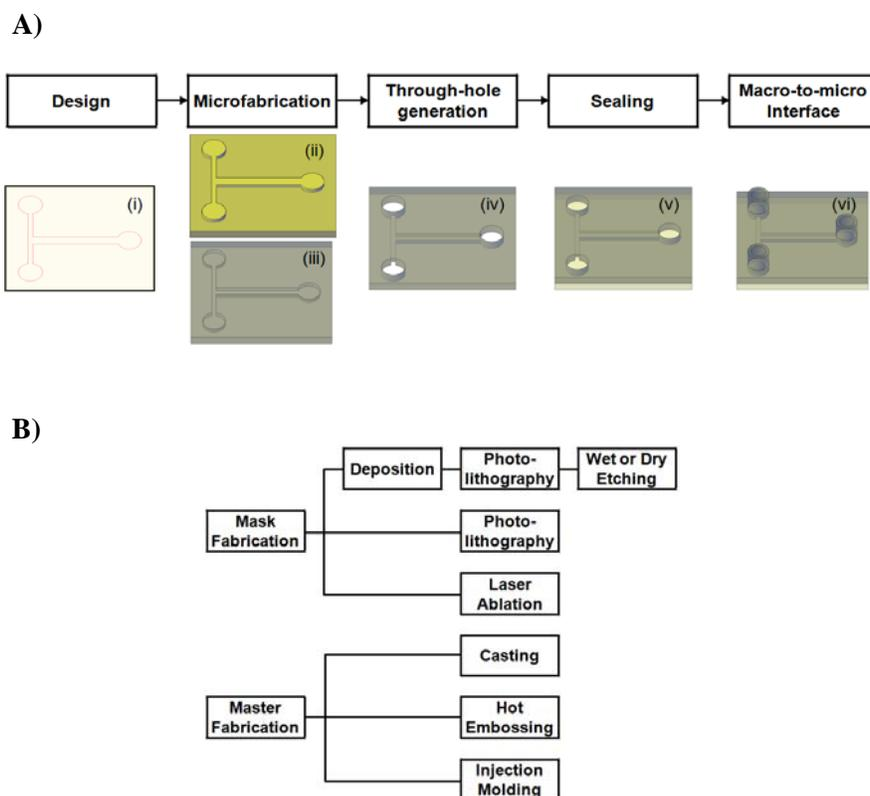
**Figure 3. A) The overall fabrication process of microfluidic devices: i) design of a microfluidic device, ii) fabrication of a master mold, iii) fabrication of a microfluidic device, iv) generation of through-holes, v) sealing, and vi) incorporation of macro-to-micro interface. B) The steps in microfabrication processes commonly used for fabrication of microfluidic devices.**
