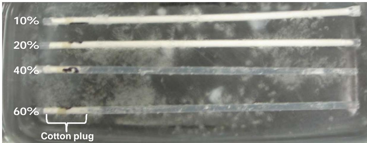
**Figure 3. Visual observation of crystallization and vitrification of ethylene glycol at different concentrations. French straws (0.25-ml) with a cotton plug at one end were filled with 10, 20, 40 or 60% of ethylene glycol and plunged into liquid nitrogen. Straws with 10 and 20% had a milky appearance indicating ice formation while straws with 40 and 60% remained transparent indicating glass formation.**
