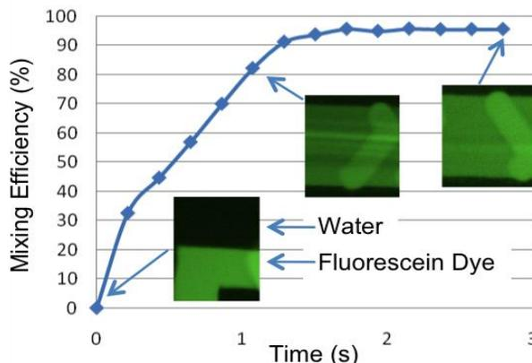
**Figure 7. Mixing of fluorescein and water across herringbone mixing elements occurred in less than 2 sec (at 100  $\mu$ l/hr) in the prototype design.**
