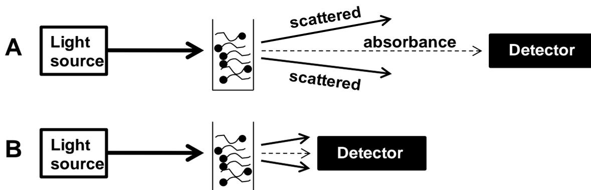
**Figure 2.** The measurement of absorbance varies depending on position of the detector. For accurate measurement it is necessary to eliminate or minimize the effect of light scattering. **A)** Positioning of the detector far from the sample enhances sensitivity because it will detect less scattered light. **B)** When the detector is close to the sample, scattered light will cause an artifactual reduction of absorbance (modified from Poole and Kalnenieks 2000).
