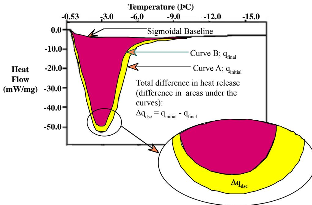
**Figure 1.** Superimposed heat flow thermograms measured by DSC obtained during the *initial* (Curve A) and *final* (Curve B) cooling runs. The negative axis for the heat flow on the y-axis implies an exothermic heat release in the DSC sample. The heat flow (mW/mg) is plotted along the y-axis and the subzero temperatures ( $^{\circ}\text{C}$ ) are plotted along the upper x-axis.
