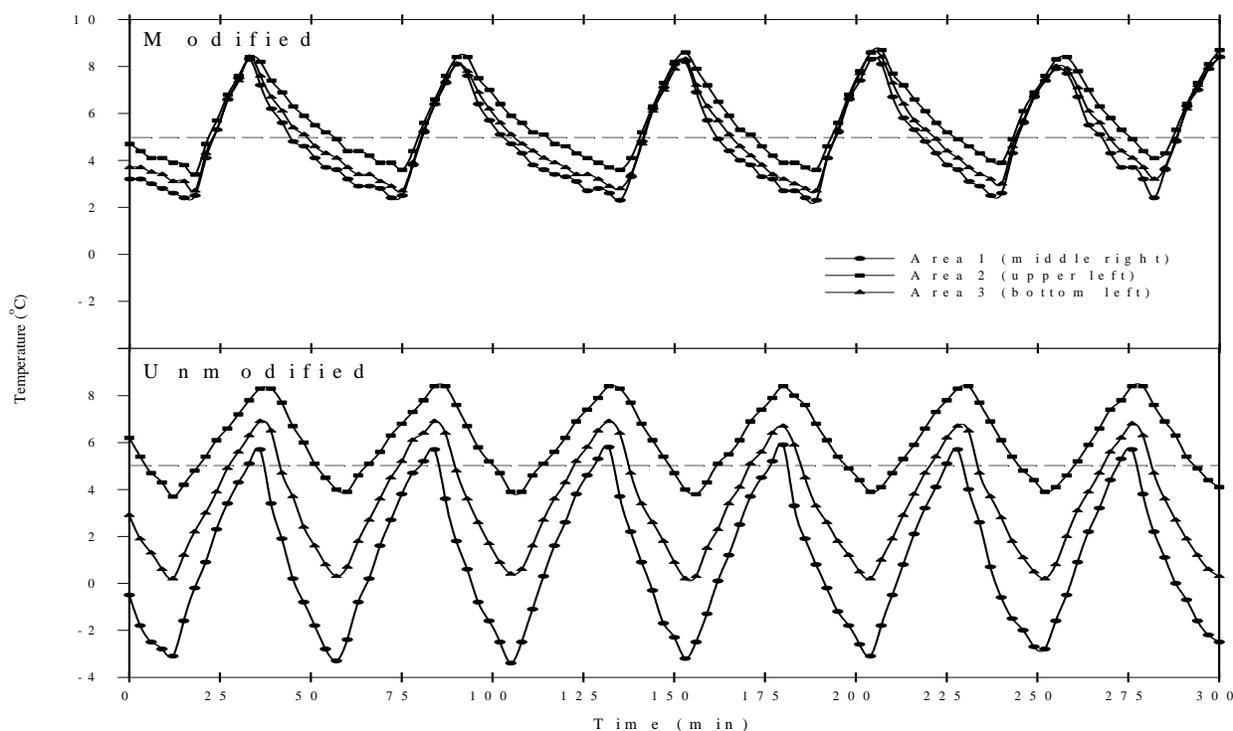
**Figure 2. Comparison of spatial variation in temperature in modified and unmodified incubators set at 5 °C. Temperatures were recorded for three areas within the incubator: Area 1, middle, right (below the freezer compartment); Area 2, upper left, and Area 3, bottom left.**
