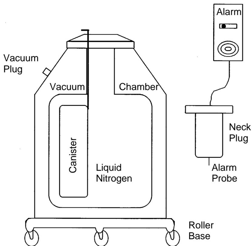
**Figure 4. Diagram of a LN<sub>2</sub> storage dewar.**
