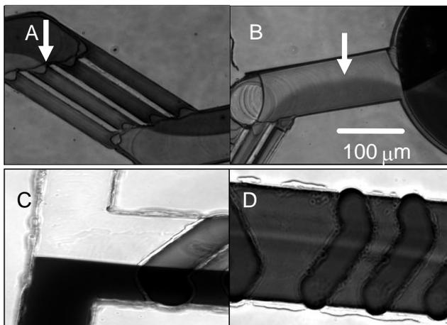
**Figure 5. Multiple intersecting zigzag microchannels (A-B) and herringbone mixers (C-D) for mixing in a microfluidic channel. The herringbone design provided more complete mixing by the end of the microchannel (D) than did the multiple intersecting zigzag design (arrow indicates unmixed fluid in B).**
