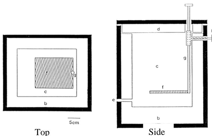
**Figure 1. Insulated freezing box used for cryopreservation of salmonid semen. Scheme: a) exterior wall; b) insulating layer; c) freezing chamber; d) cover of freezing box; e) overflow trap for LN<sub>2</sub>; f) platform for straws; g) attachment bar of platform; h) set screw.**
