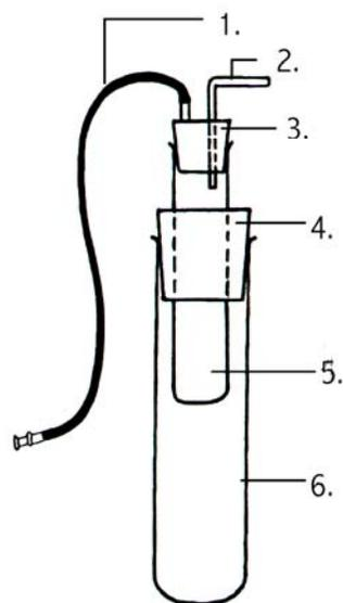
**Figure 1. Salmonid milt aspirator: 1) 0.3 cm ID × 0.5 cm OD latex tubing; 2) 2.2mm ID × 3.2 mm polyethylene tubing; 3) two-hole “O” stopper; 4) # 6 ½ stopper bored with a # 6 borer; 5) 14-mL graduated Falcon tube; 6) polycarbonate round-bottom centrifuge tube (100 mL, 31.5 mm × 166 mm).**
